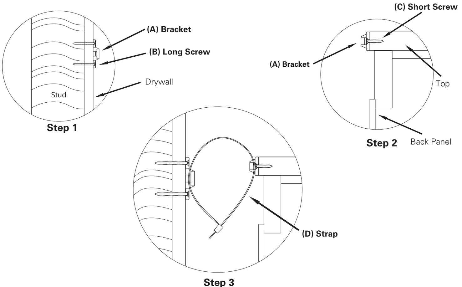
**A.** Locate a stud in the wall behind the dresser. {The stud is the solid wood piece that supports the wall-you must screw into a solid support, and not directly into drywall.} Position a bracket (A) on the stud slightly below the top of the furniture. Mark and drill a hole into the center of the stud using a 3/32" drill bit. Attach the bracket to the stud with the long screws (B).
