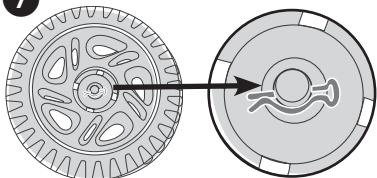
**7** Fit straight part of cotter pin through hole on axle.
