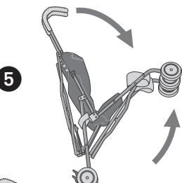
**5** Push handlebars forward and squeeze stroller together.
