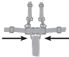
4 To fasten restraint system buckles - push together. Be sure both buckles are fastened to secure child safely.
