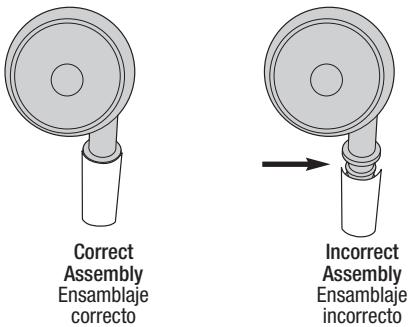
**CAUTION:** Be sure the caster is inserted fully into the base. The top lip of the caster threads should be flush with the base hole. Nothing below this lip should be visible.
