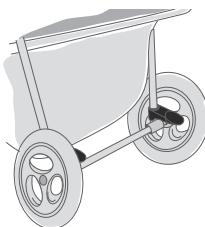
**1** Push levers on both rear wheels down to lock.
