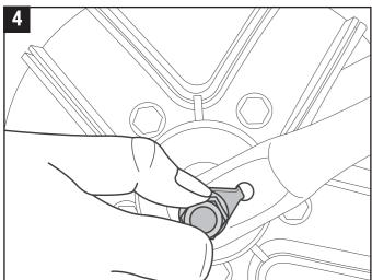
**STEP 4** - Ensure that the tab on the tear drop shaped washer is aligned with the hole on the front fork as shown. Repeat for other side.
