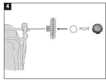
STEP 4 - TO INSTALL NEW REAR WHEEL: Put new rear wheel on axle. Slide washer onto axle. Fit straight part of cotter pin through hole on axle. Insert hub cap into wheel. Repeat Steps 2 through 4 for other rear wheel.
