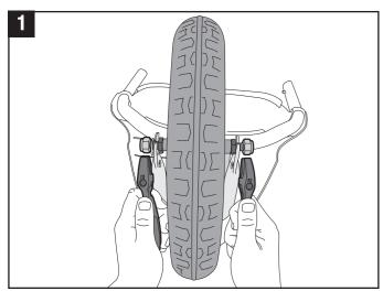
**STEP 1** - Position stroller, so that the handle and rear wheels are resting flat on the floor.
